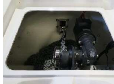
Windlass + anchor locker
