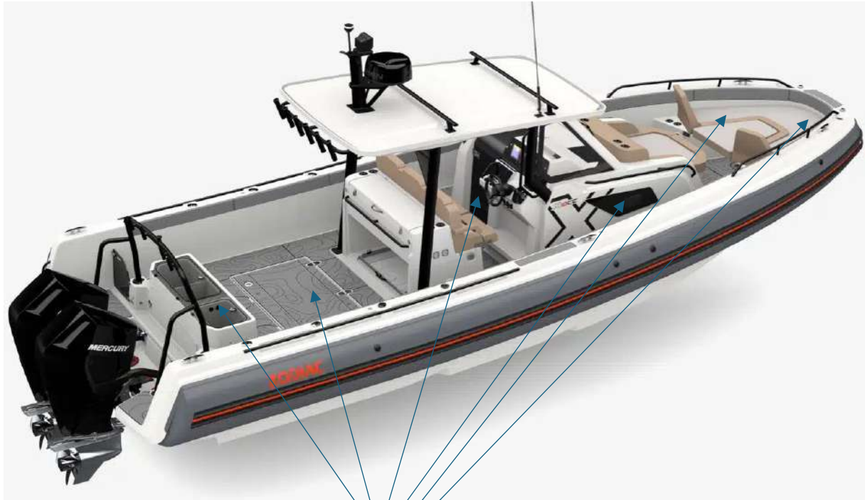
Deck hatches, openings and lockers
